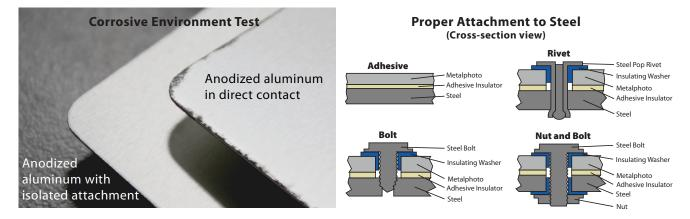
Examples of Metalphoto properly attached to steel with no corrosive degradation.
